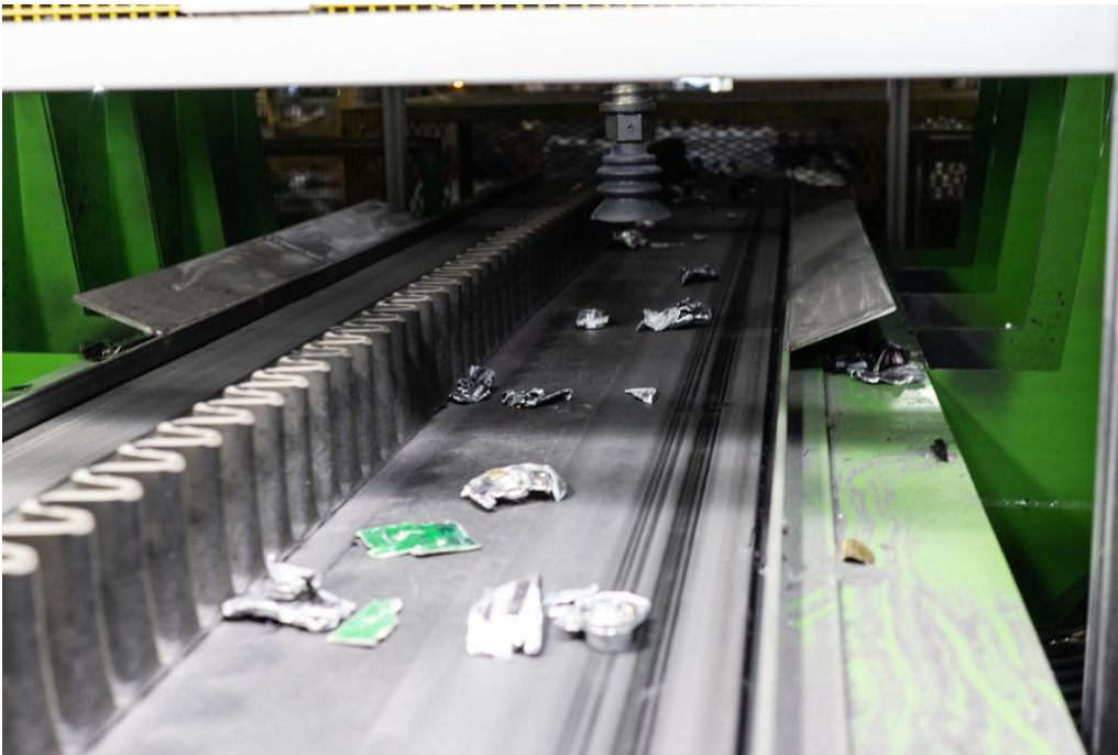
An Electronic Recyclers International shredder moves hardware along on a conveyor belt, then slices and crushes it.
